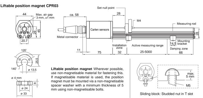
**Note:** On installation of the CARLENsensors, careful shielding from magnetic and electromagnetic fields must be ensured. The cable shield must be mounted on the connector and connected to ground at the evaluation electronics. All data sheets and manuals are also available in the Internet under **www.carlen-sensors.com**
